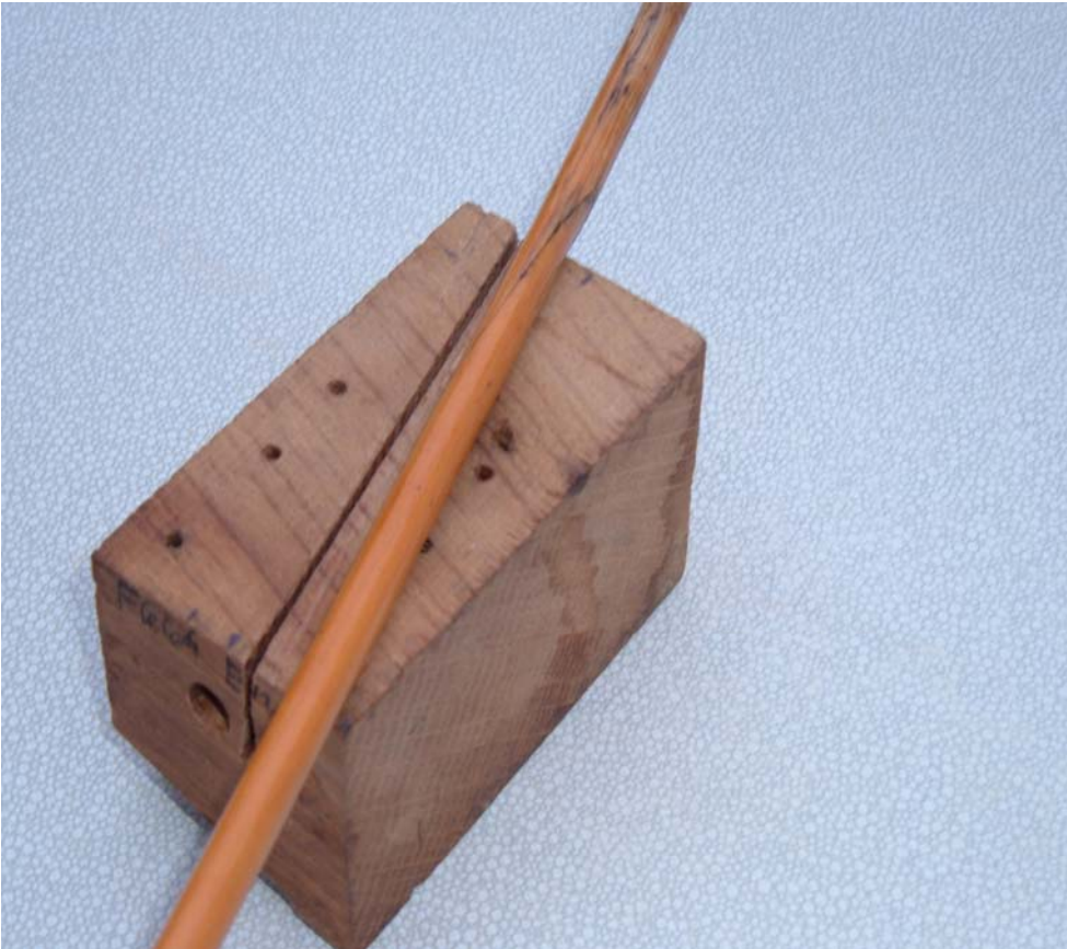
Arrow joining jig with arrow showing angle of cut.
