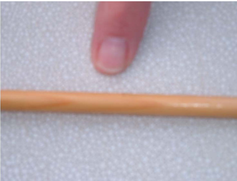
Grain breakout on the shaft of an arrow.
